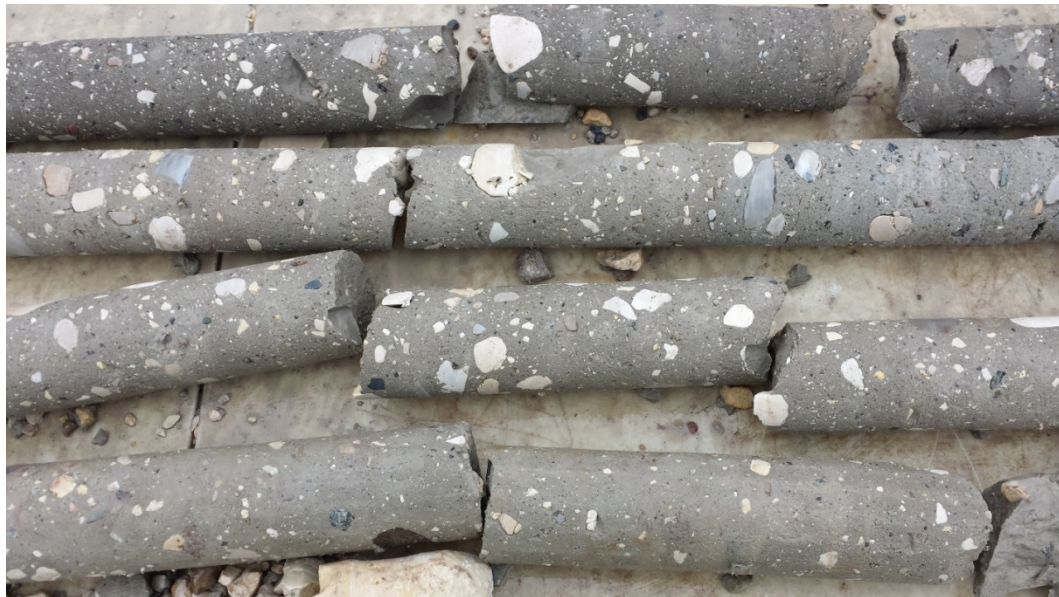
Photo D8-C6 – Example of cored and well-cemented basal till along Route D (TH-ED01). Core diameter is 63.5 mm.
