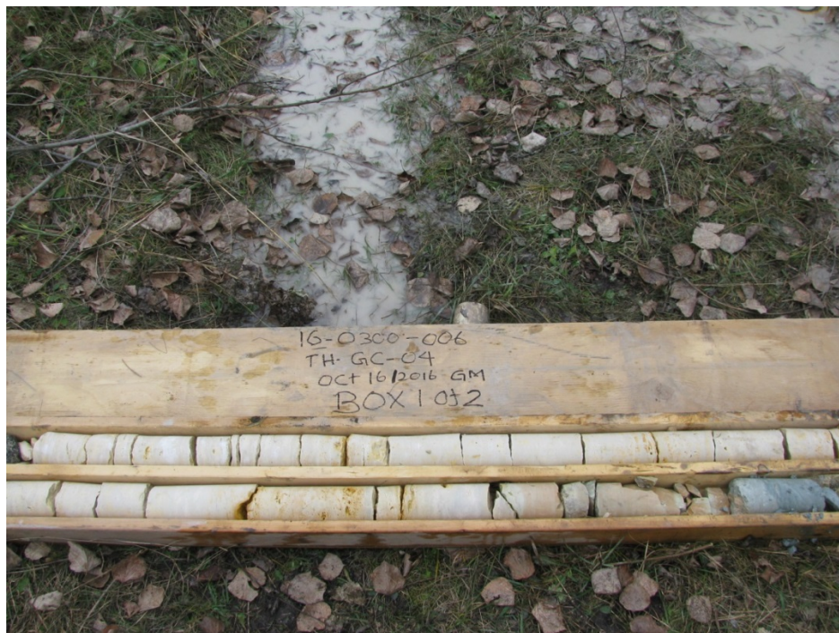
Photo D8-C4 – Example of good quality bedrock along Route C (TH-GC04). Core diameter is 63.5 mm; length of core box approximately 1.5 m.
