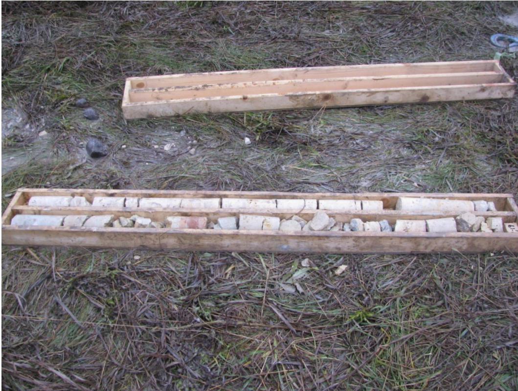
Photo D8-C5 – Example of reasonable quality bedrock along Route D (TH-GD07). Core diameter is 63.5 mm; length of core box approximately 1.5 m.
