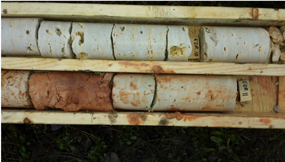
Photo D8-C1 – Example of typical vuggy core, and shale infill zone within bedrock along Route C (TH-EC01-P). Core diameter is 63.5 mm.
