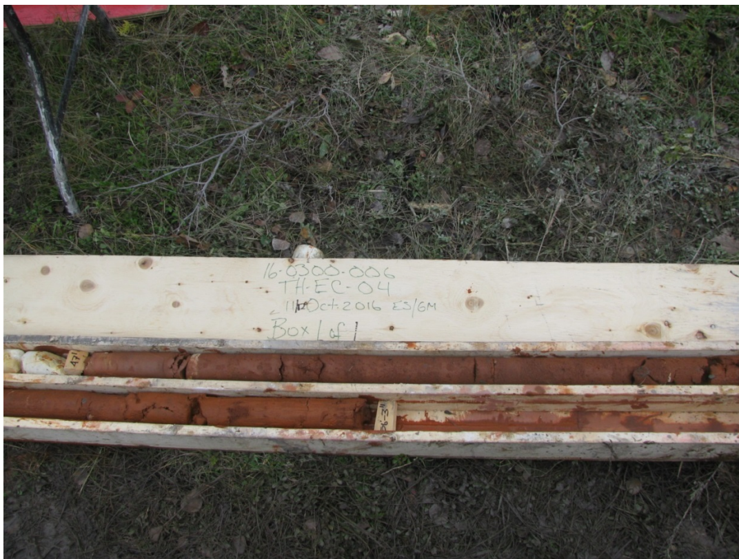
Photo D8-C2 – Extensive shale infill zone within bedrock along Route C (TH-EC04). Core diameter is 63.5 mm; length of core box approximately 1.5 m.
