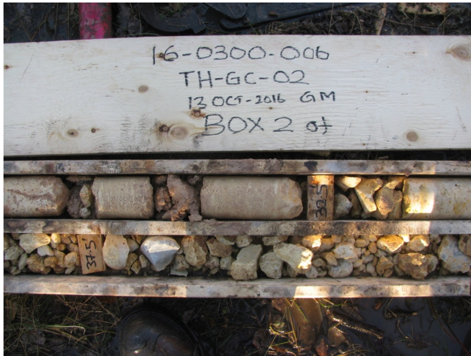
Photo D8-C3 – Example of broken core/rubble zone within bedrock along Route C (TH-GC02). Core diameter is 63.5 mm.
